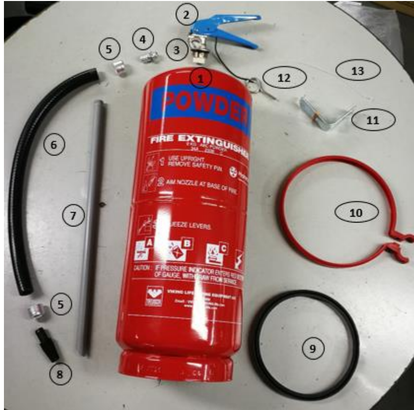
Figure 1: Dismantled 6kg Powder Cartridge Operated Fire Extinguisher
